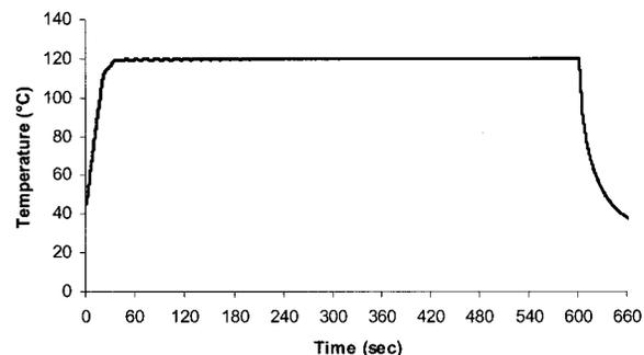
**Figure 1.** Heating profile for a typical Biginelli condensation in AcOH/EtOH (3:1) under sealed vessel/microwave irradiation conditions: microwave flash heating (300 W, 0–40 s); temperature control using the feedback from IR thermography (constant 120 °C, 40–600 s); active cooling (600–660 s).
